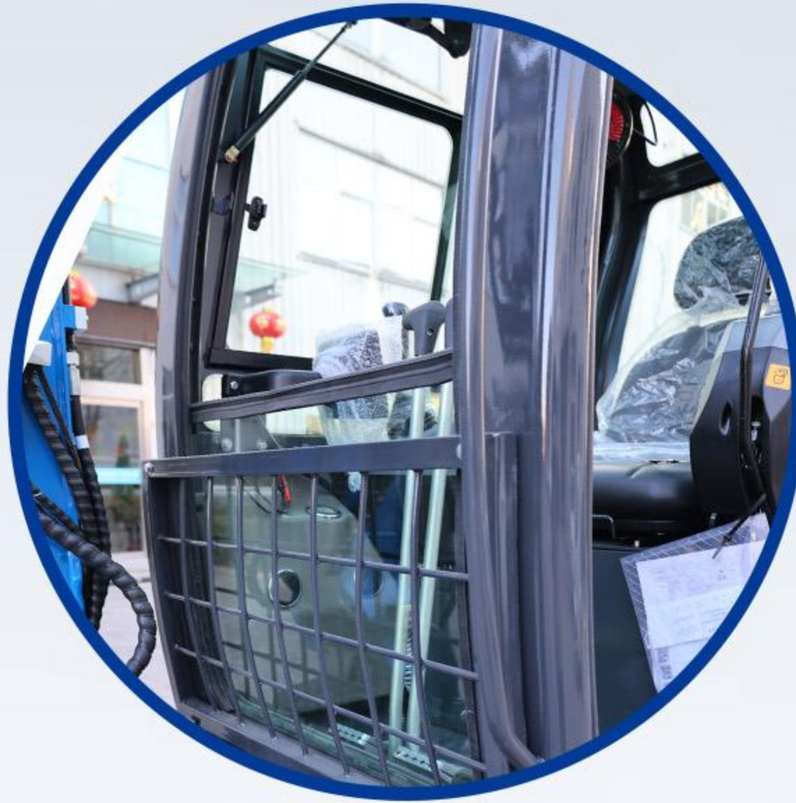
Flip-up front glass + pro- tective net
