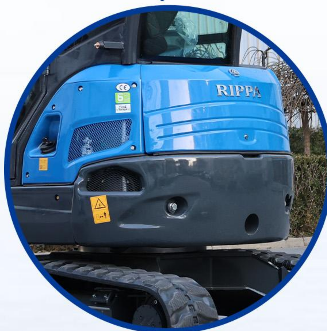
Counterweight-Real weight : 3.2Ton
